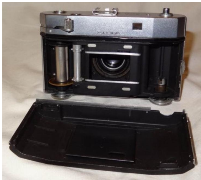
Rear view of Fenix series "a" with rewind fork
