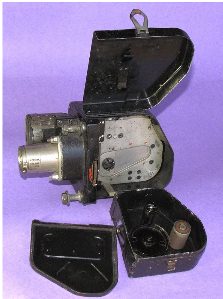
Internal view of the chamber in Polish S-13
