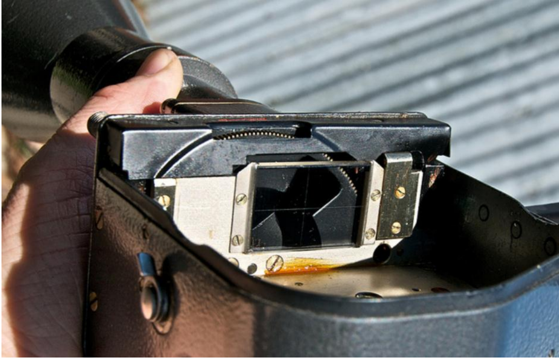
Openings shape in the S-13 high speed rotary focal plane shutter
