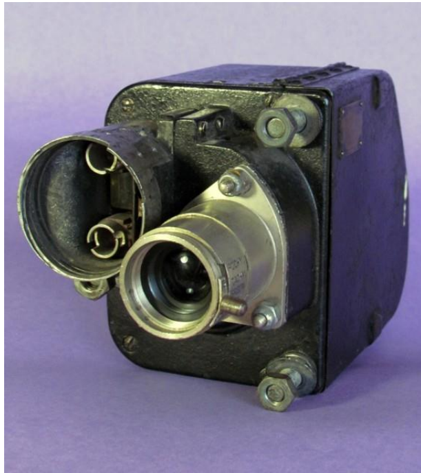
Polish version of Soviet S-13 aerial camera
