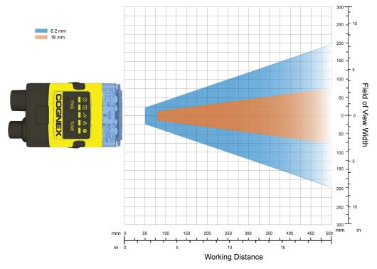
The following chart shows the horizontal field of view for In-Sight 2000 Mini vision sensors with 640 x 480 image resolution (2X Image Magnification mode).
