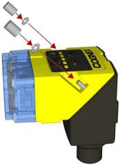
7. After each cap nut has been fastened, torque to 0.12 Nm (1.06 in-lb) and reinstall the screw covers.
