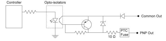
When connected to the CIO-1400 I/O expansion module, the two high-speed outputs are configured as NPN (current sinking) with 50mA maximum current and the general-purpose outputs are configurable as NPN (current sinking) or PNP (current sourcing) with 100mA maximum current.
