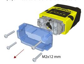
3. Insert the filter at the bottom side of the round opening in the transparent plastic part.
