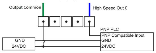
To connect the high-speed outputs to a relay, LED, or similar load, connect the negative side of the load to the output and the positive side to +24VDC. When the output switches to ON, the negative side of the load is pulled down to less than 3VDC, and 24VDC appears across the load. Use a protection diode for a large inductive load, with the anode connected to the output and the cathode connected to +24VDC.
