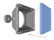
5. Reinstall the filter holder back to the cover. Tighten the screws until they stop turning.
