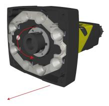
5. Insert the new lens and using your fingers, turn it clockwise to tighten the lens.
