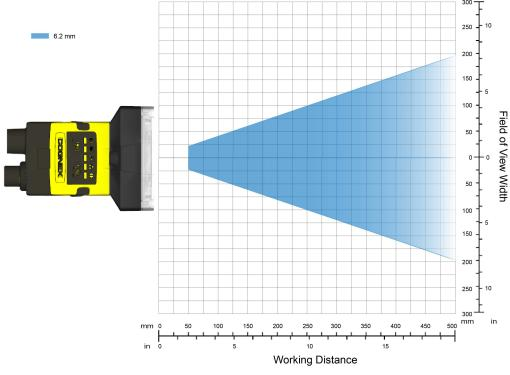
The following chart shows the horizontal field of view for In-Sight 2000 vision sensors with 640 x 480 image resolution (2X Image Magnification mode).
