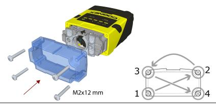
(i) Note: The rib in the front cover must be oriented to the top side.
