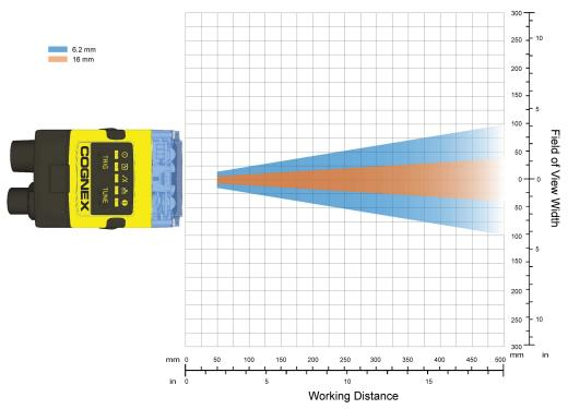
The following chart shows the horizontal field of view for In-Sight 2000 Mini vision sensors with 800 x 600 image resolution (2X Image Magnification mode).
