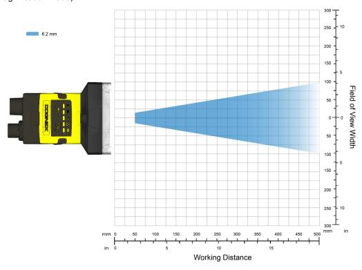
The following chart shows the horizontal field of view for In-Sight 2000 vision sensors with 800 x 600 image resolution (2X Image Magnification mode).
