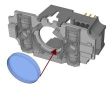
4. Push the top side of the filter firmly until it is sitting flat against the PCB.
