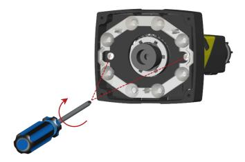
7. Reattach the cover. Tighten all four screws using a torque wrench; the maximum torque is 0.2 Nm (1.77 in-lb).
