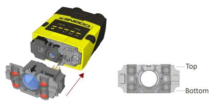
5. Attach the cover. Observing the tightening sequence below, tighten all four screws to 9 Ncm (0.80 in-lb) using a torque wrench.
