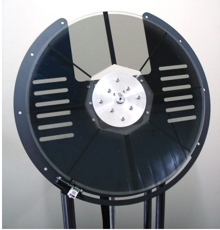
[Picture 5] After removing the safety cover of circular polarized rotary filter
