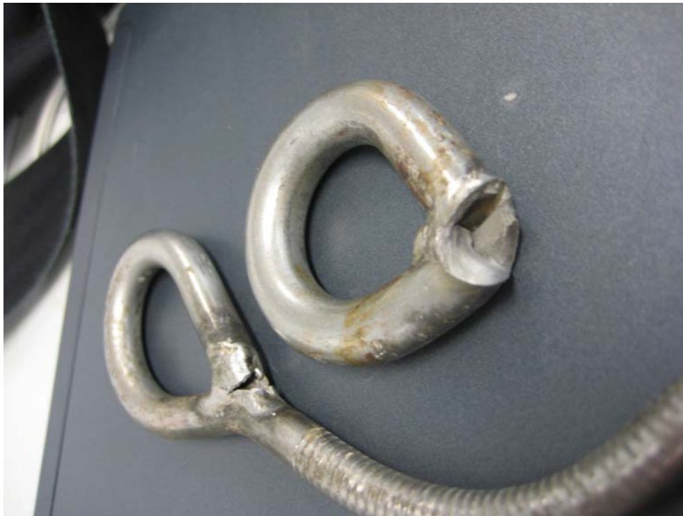
Figure 1.8 Weld failure in 8mm tested ring. Snapped 10 mm ring, snapped by hand force of ~ 10kg with a 150mm shifter.
