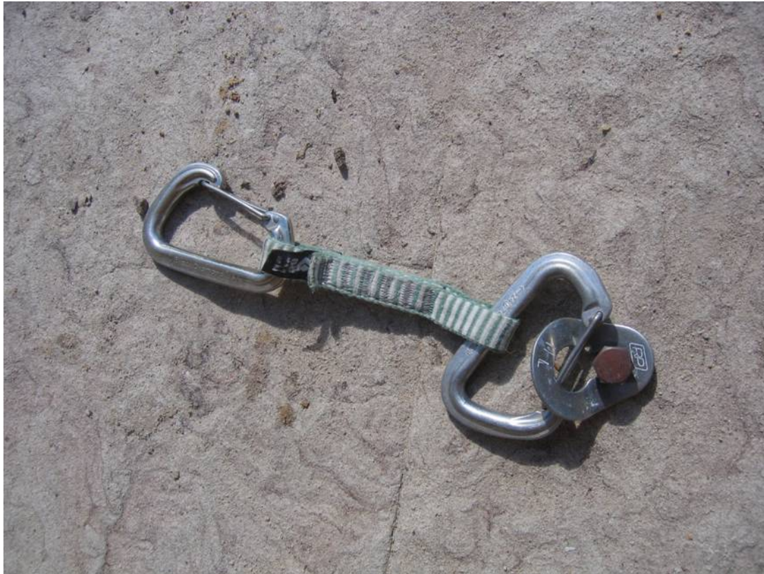
Figure 6.2 Wire gate flipped sideways for automatic self soloing. The gates are very weak in this configuration also.
