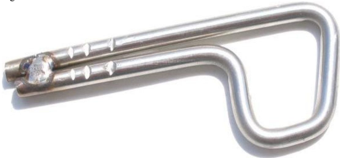
Figure 1.3 10cm Buhler bolt with less welding and some notches
