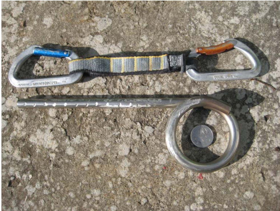
Figure 1.9 Massive 13 mm rod welded ring with 230 mm embedment. Probably bomber.
