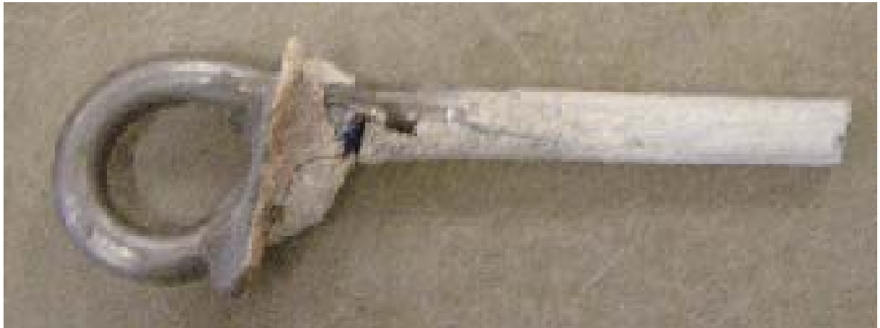
Figure 3.2 Rock and bond failure. In this case the depth of the cone is approximately 20mm and the length of bond failure is 100mm. Polyester glue was used, which has about half the strength of epoxy. As we show later, the use of a stronger glue will increase both the length of the failure cone, and also increase the failure load.
