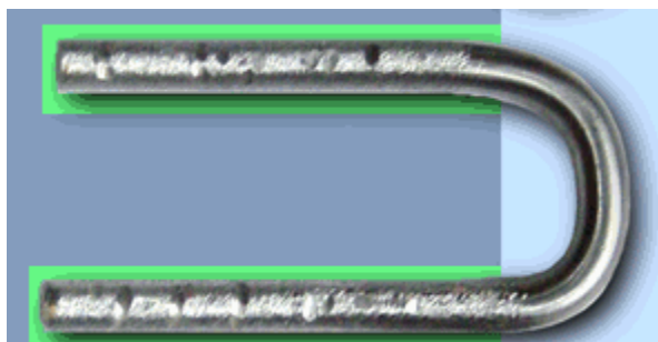
Figure 7.1 Typical homemade Ubolt showing grinding, notching, and reduced eye profile
