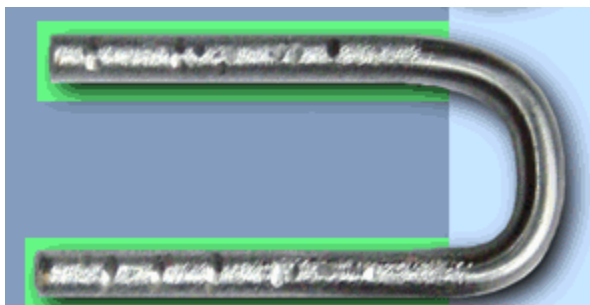
Figure 1.7 Typical homemade Ubolt showing grinding, notching, and reduced eye profile. 90 mm embedment and 40 mm spacing.
