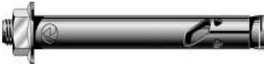
Figure 4.3 Dynabolt – 10 mm diameter is good in strong rock
