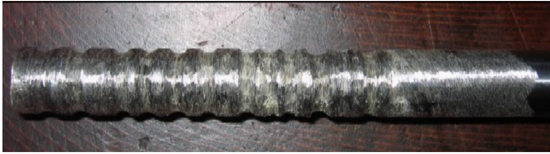
Figure 2.7 Rotary notch method
