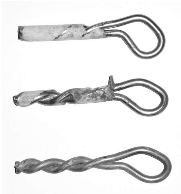
Figure 2.1 Top - Hole blown out with blower. 10.4kN. Centre - Hole blown out with compressed air at 8 bar. 15.3kN. Bottom - Hole blown, brushed and blown with blower. 34.7kN - From Bolting Products
